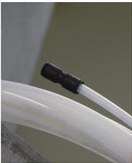
This black plastic push connector is fine for a monitoring line but not durable enough for introduction. Failure of a similar connector resulted in the blowout shown in the photo above.
